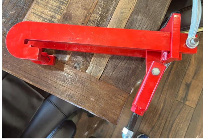
Figure 3. Bobby Jack OPS (offset pipe support).
